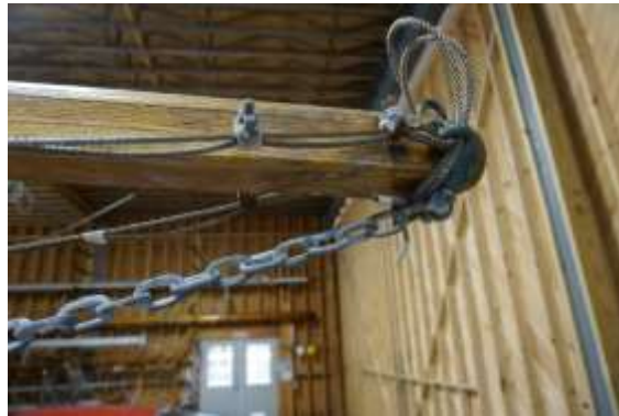
Figure 10.20 Cable clamps on bowsprit rigging
