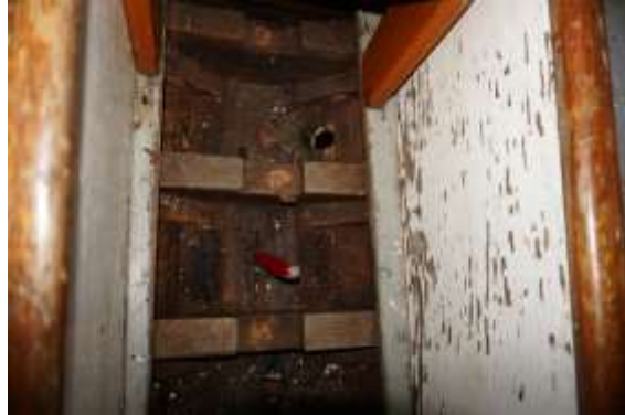
Figure 10.14 Rot pocket in top of keel
