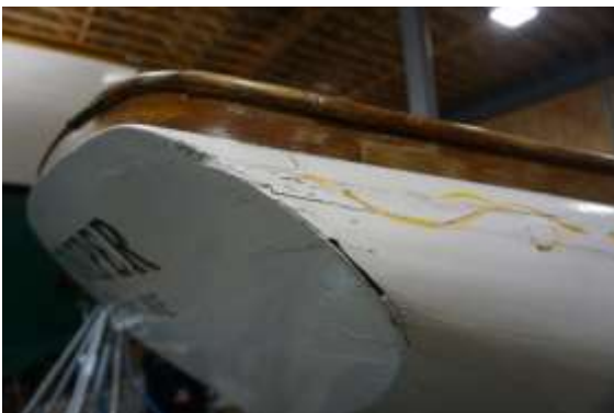
Figure 10.17 Dry planking on transom hood-ends
