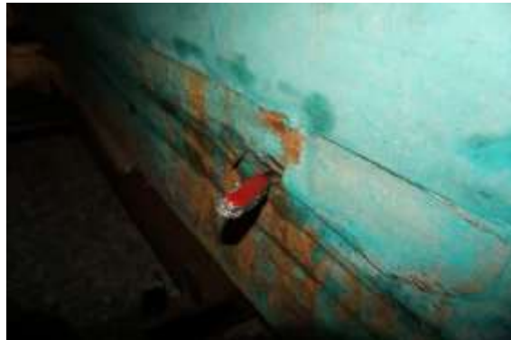
Figure 10.16 Rot pocket in keel
