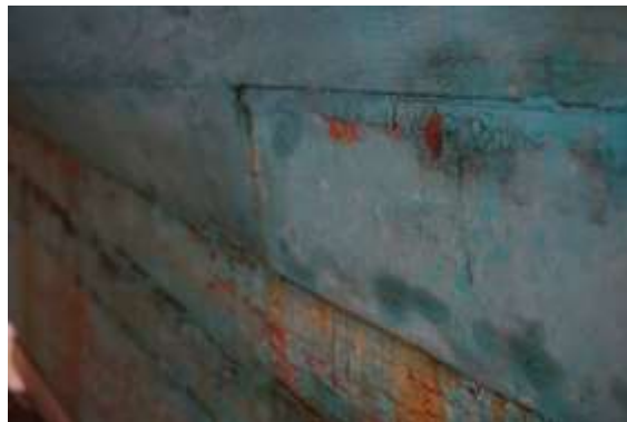
Figure 10.22 Set in garboard plank at butt
